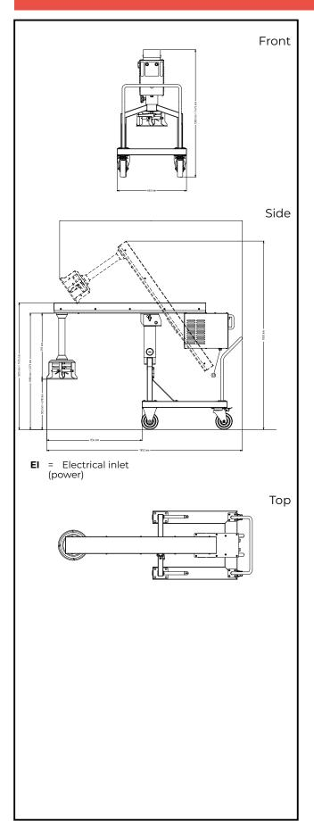
Electric Supply voltage: 380-415 V/3 ph/50 Hz Electrical power, max: 4.5 kW **Total Watts:** 4.5 kW Capacity: Capacity (up to): 1000 Litre Key Information: External dimensions, Width: 663 mm External dimensions, 1852 mm Depth: External dimensions, 1475 mm Height: **Shipping weight:** 220 kg
